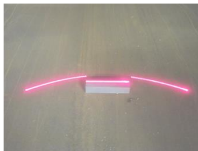
Figure 3: Laser Line projected at angle on surface of the pipe
